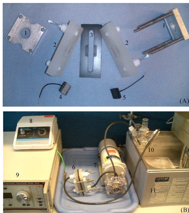
Fig. 1. Photographs showing (A) flow cell components and (B) assembled flow cell system. (1) Cell clamp; (2) flow compartment plates; (3) gasket and interelectrode spacer; (4 and 5) electrodes; (6) assembled flow cell; (7) peristaltic pump and pump head; (8) pump controller; (9) potentiostat/galvanostat; (10) electrolyte reservoir; (11) thermostated water bath.
